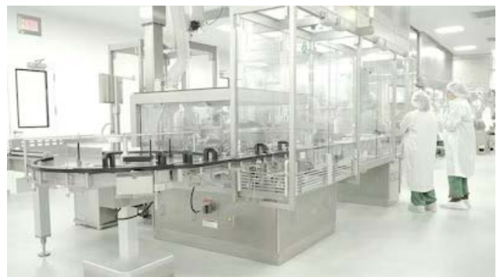
groninger integra vial filling line with SKAN isolator.
