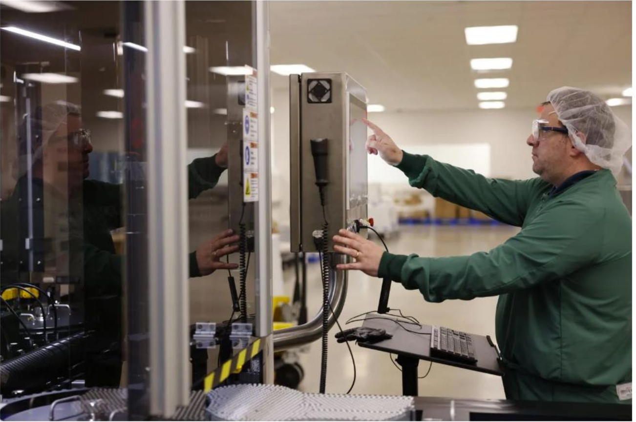
A Civica employee operates a machine that checks vials of insulin for leaks, seal defects and foreign particles on Dec. 20 in Petersburg.
